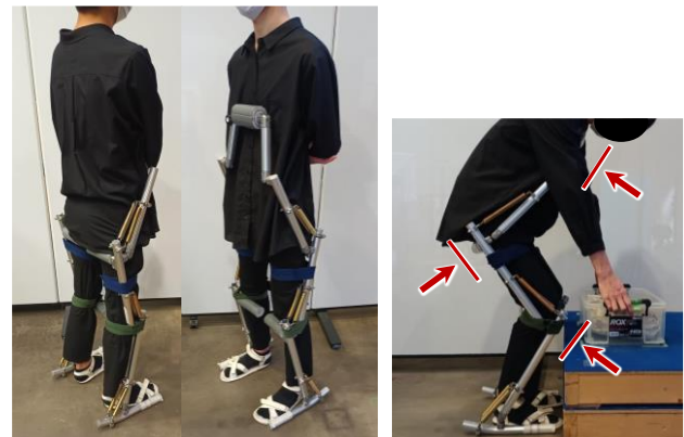
Figure 1 The prototype exoskeleton. It supports part of the body weight as indicated by the arrows and assists bent posture and extensions of the lower back and the lower limbs.
